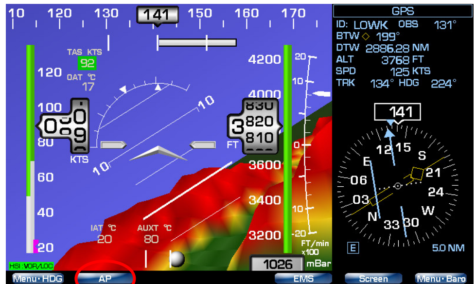
EFIS/GPS screen when Towing Menu is OFF
